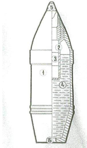
Figure 1. Russian chemical projectile 1. Body, 2. explosive well 3. explosive charge 4. fuse, 5. filling plug
