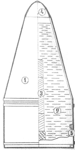
Figure 2. Russian chemical warhead for tactical missile. 1. Body, 2. chemical agent, 3. explosive charge, 4. fuze, 5. filling plug It contained 555 kg VX
